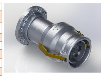
The main parts of the coupler are made in aluminium alloy. Standard seals in hydrogenated Buna (HNBR) are easy to maintain. The surfaces subject to wear are hard coated.
