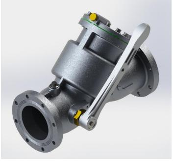
The main parts of the coupler are made in aluminium alloy. Standard seals in fluoroelastomer FPM-NT (Viton®) are easy to maintain. The surfaces subject to wear are hard coated.
